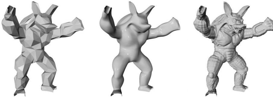
Figure 13.51: To the left is a coarse mesh. In the middle, it is subdivided using Loop's subdivision scheme. The right image shows the displaced subdivision surface. (Image courtesy Aaron Lee, Henry Moreton, and Hugues Hoppe.)
