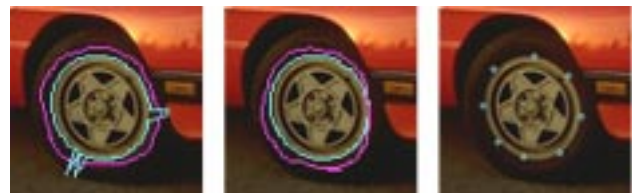
Figure 10: Circling the wheel. The counter-clockwise path of the pointer is shown in magenta, the path of the cursor in cyan. If the user is not careful, lack of hysteresis can cause bad snaps during circling, as seen on the left. The center shows a more careful tracing. The right shows an alternate interaction technique: the user specifies discrete points through which a curve will be fitted.
