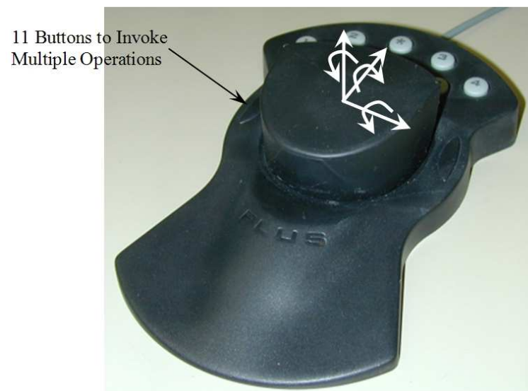
Figure 5.7 3D mouse and its functionalities in the 3D mode
