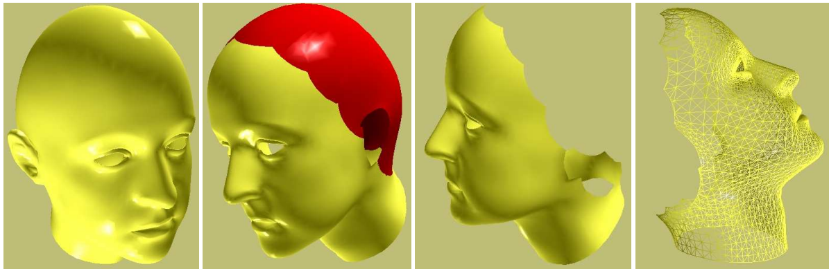
(a) imported surface model that (b) thick-brush tracing was done to (c) traced region is erased from the (d) resulting final geometry rendered in wire-frame mode was modeled in another model- select a region of the model (shown surface geometry ing system in red)
