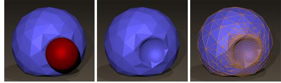
**Figure 7:** (Left) A coarse deformable ball collides with a kinematic sphere. (Middle) Soft bindings enable subtetrahedron elasticity in response to the collision. (Right) The dynamically refined surface mesh.
