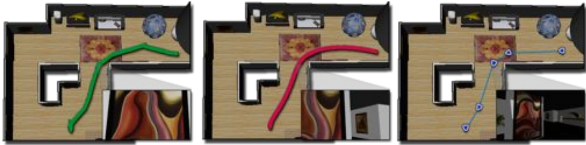
Fig. 1. Viewpoints in camera paths. The green path, shown on the left, corresponds to the original motion of 1,400 viewpoints. The pink path in the middle demonstrates that the filtered path, while smooth, does not show all of the items seen in the original path. The extracted path, shown in blue on the right, comprises five viewpoints that demonstrate the views seen in the original path.
