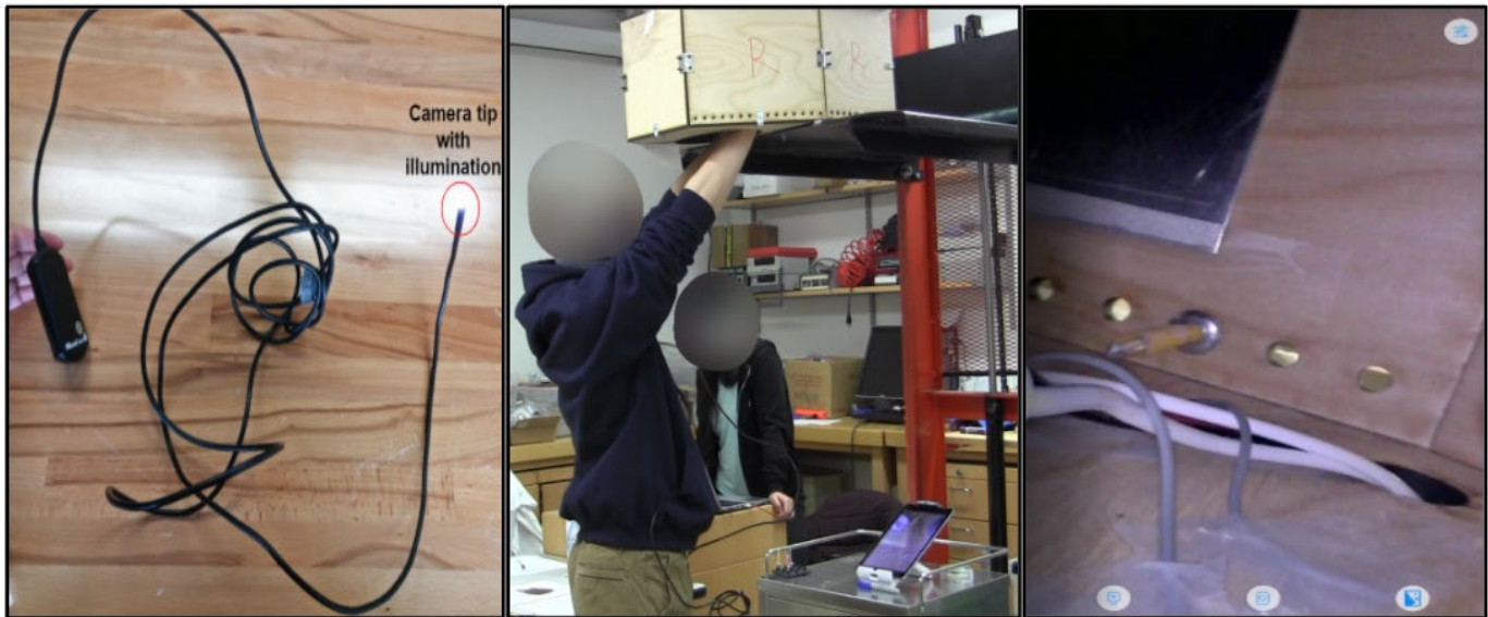
Figure 3. (a) Borescope. (b) Participant using the borescope for the second rivet insertion task. (c) A view from the manufacturer's application during the second rivet insertion task showing the yellow rivet inserted into the third hole from the right, as instructed to the participant
