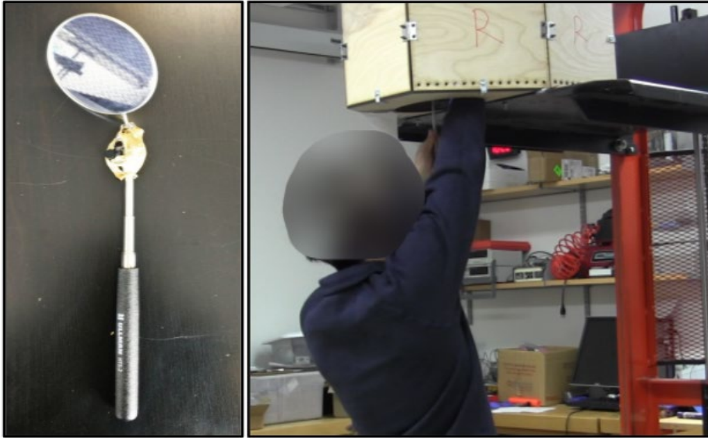
Figure 2. Mirror with additional LED light, participant using the mirror for the first rivet insertion
